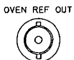
Supplies a 10 \text{ MHz} \pm 1 \times 10^{-7} per month sinusoidal frequency reference from an internal crystal oscillator, located in a temperature-controlled oven. The output is ac coupled and the output impedance is 50 ohms. The nominal output level is +10 dBm/50 ohms. The output is disabled during the oven's warmup cycle. To use the internal Oven Reference, this output must be connected to the EXT REF IN jack.
